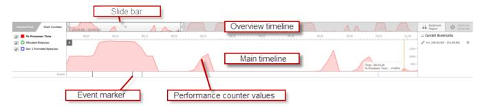
The overview timeline shows performance data for the whole profiling session. To minimize the timeline so that only the overview is visible, click Collap se on the Timeline bar (ANTS Performance Profiler 8.6 and later).
