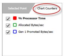
The Chart Counters tab shows all your counters, and lets you highlight one as a main counter. The main counter is shown as a filled box, and the area under its graph is shaded on the timeline. Other counters are shown with an unfilled box in the Chart Counters tab and by colored lines on the timeline.
