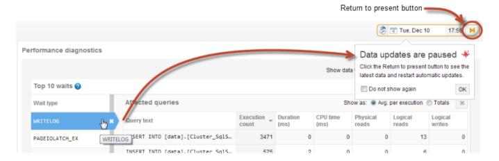
Data will remain frozen until you click the Return to present button. For more details about the Back in Time control, see Rewinding time with Back in Time mode.
