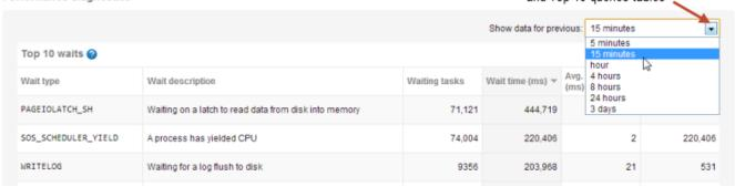
You can also display data from a previous time period of your choice using the Back in Time control. For more details, see Rewinding time with Back in Time mode.
